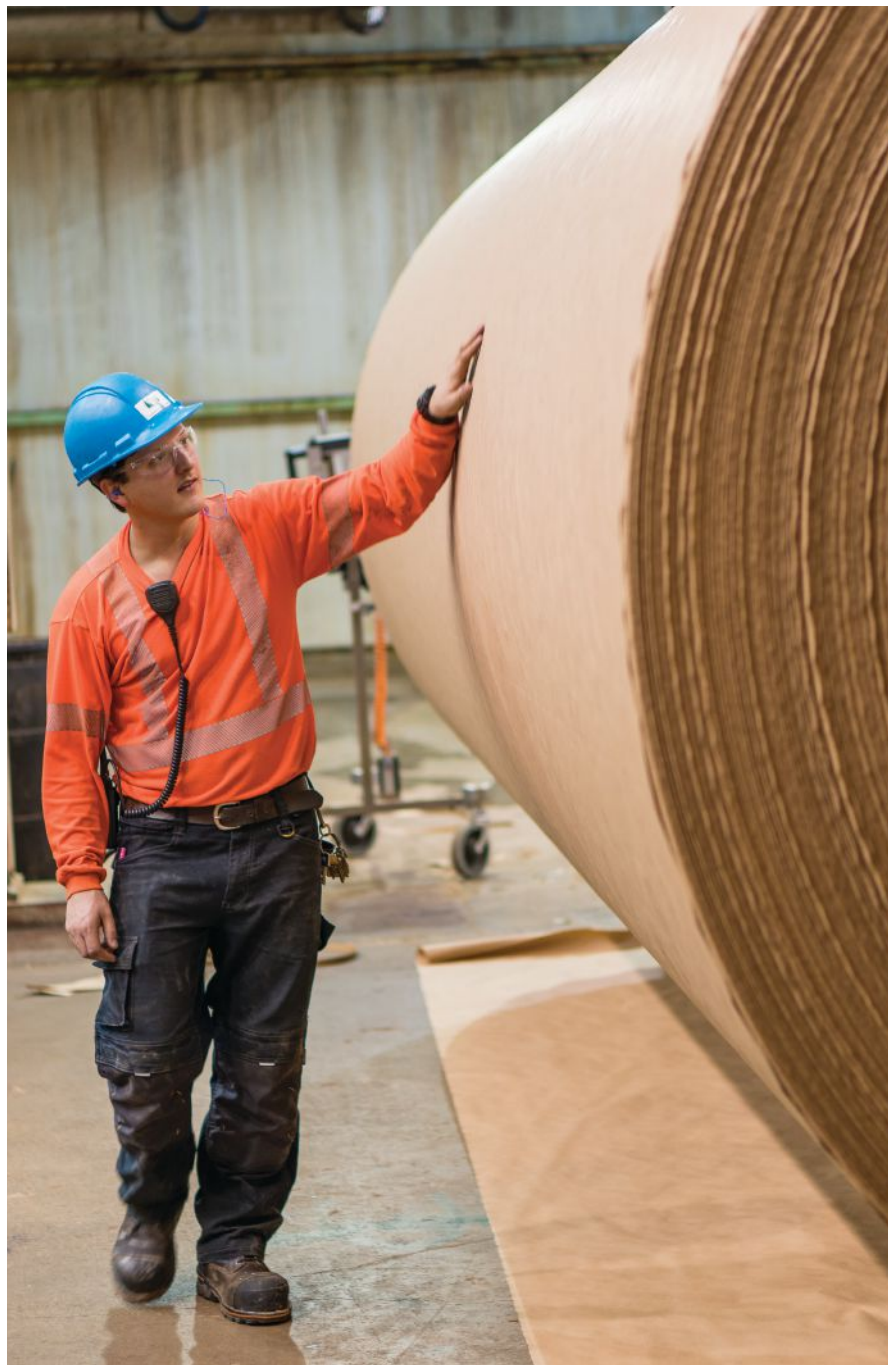
Canadian Kraft Paper manufactures its paper using 100 per cent virgin fibre, which provides strength for end uses such as heavy-duty bags.
