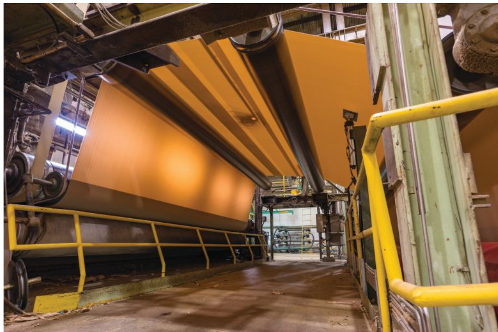
Canadian Kraft Paper operates a single production line that sees about 2,500 cubic metres of chips per day processed into unbleached sack kraft paper.
